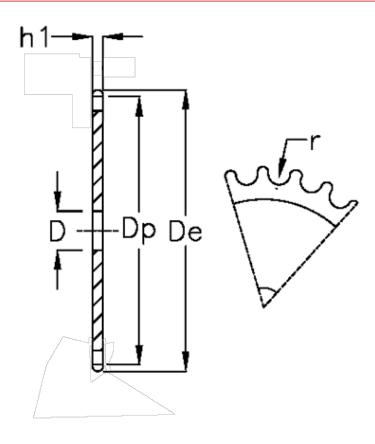
C = 1 D = 10 De = 73.6 Dp = 69.11 For chain size = 1/2 x 5/16 For chain type = 08 B-1 h1 = 7.2
